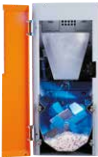
Weigh bin and mixing chamber
